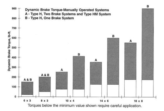
The chart below shows the dynamic torque ranges developed by air powered hydraulic systems.
