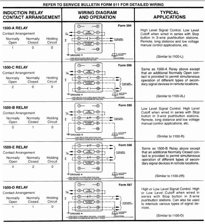
CAUTION: Electrodes are terminals of live electrical circuits and must be installed to prevent accidental contact by personnel. Control power must be disconnected before servicing.
