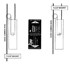
The Type C Switch is shown. It attaches to the common wire with a spring clip.
