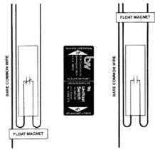
The Type I switch is shown. It attaches to the common wire with plastic tape.
