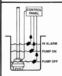
BIW Controls can provide the complete control system for a multiple float application including NEMA 1, 4 or 12 enclosures, disconnect switch, control transformer, relays, motor starters, alternators, alarms, etc.
