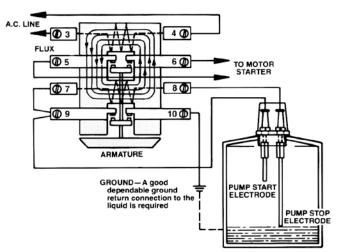
Figure 1 - Secondary coil circuit open; armature down.
