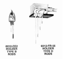
TYPE B electrode rods are 1/4" diameter and are tapped 6-32 for use only on Type CE-2 and CE-3 holders. Lengths over 12 inchs should be insulated and lengths over 30 inches are not recommended.
