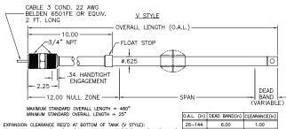
EXPANSION CLEARANCE REQ'D AT BOTTOM OF TANK (V STYLE): MIN. CLEARANCE = (0.A.L.) X (MAX. OPERATING TEMP(C) - 20) X (.00014) OVERALL LENGTH = INSERTION LENGTH - CLEARANCE + 1"
