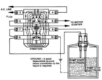
Figure 2—Secondary coil circuit closed; armature up.
