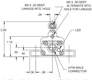
A standard 12 mm 4 pin micro connector is used. Straight mating cables can be ordered in a 6' length, or 12' length. If space is a consideration a right angle connector is also available.
