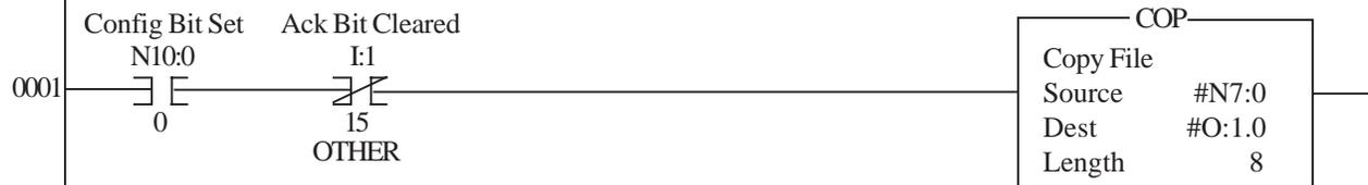
When the 1746R configuration command is complete, the program will copy the position scaling command for resolver 1 into the output image table with the programming bit set. This command will configure resolver 1 for a total scale factor of 1000 and turn count of 10. This will configure the resolver for 100 counts per turn. This continues until the command has been acknowledged.
