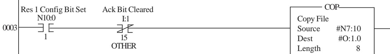
When the position scaling data has been acknowledged for resolver 1, the program will copy the position scaling command for resolver 2 into the output image table. This resolver is set up for a scale factor of 360 with no turns counting. This will continue until the command has been acknowledged.
