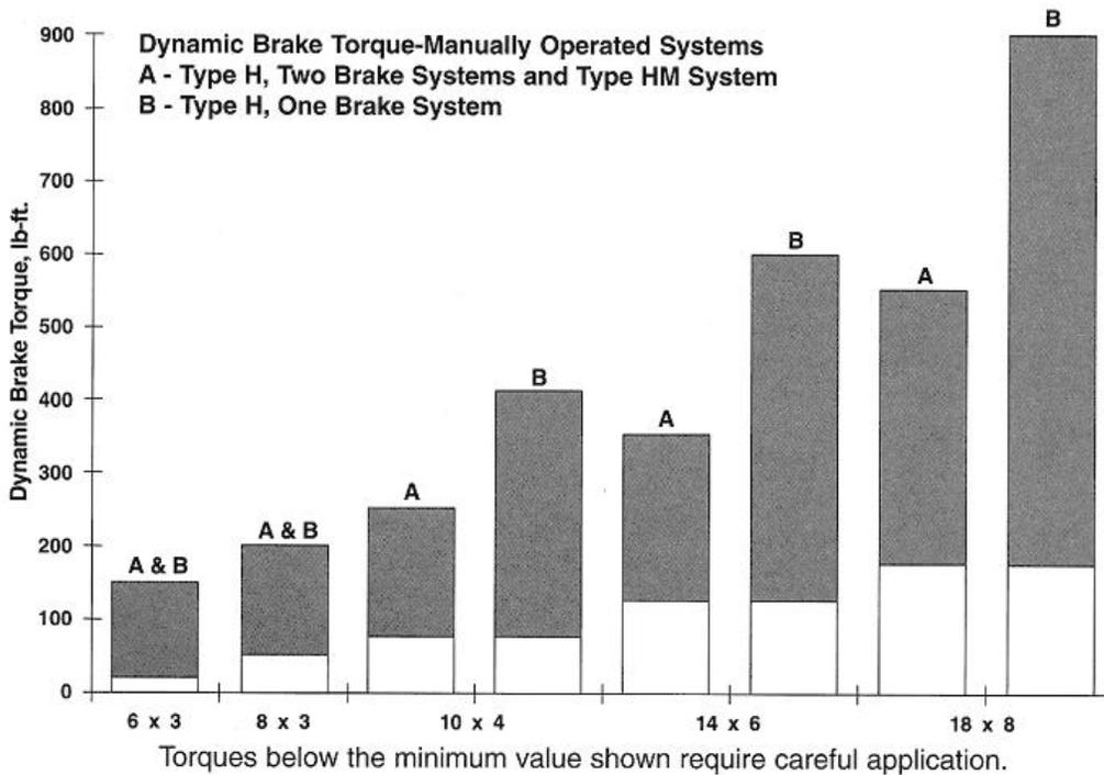
The chart below shows the dynamic torque ranges developed by air powered hydraulic systems.
