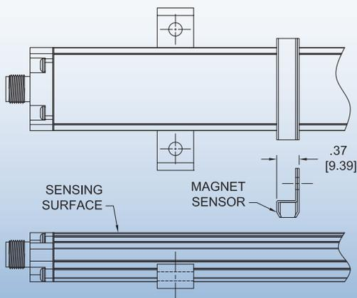
All units are provided with mounting feet and a magnet assembly. The mounting feet (SD0522000) slide in the grooves on the side of the extruded housing. When tightened down with fastening hardware, the mounting brackets clamp the unit into place.
